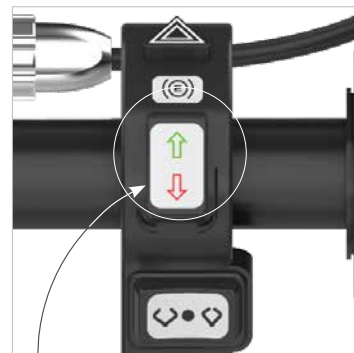
Forward and reverse gear
